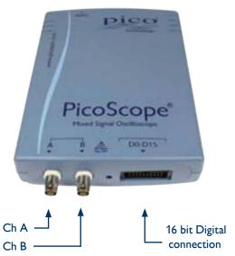
The front panel of the PicoScope 2205 MSO has two BNC analog input channels and a connection for up to 16 digital signals.
