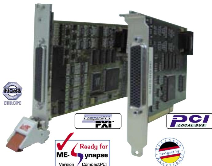
**Versatile analog output board at a reasonable price: This solid standard D/A board gives you up to 16 voltage outputs with 12 bit resolution. On the model "UI" you can also use 8 of the lines for current output, if required. The current ranges are 0...20 mA and 4...20 mA.**
